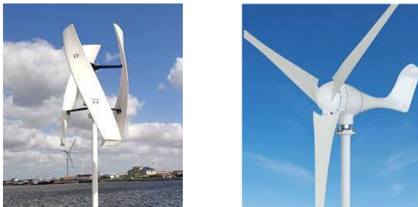
1-rasm. Vertikal va gorizonttal shamol turbinalarining ko‘rinishi [2]
